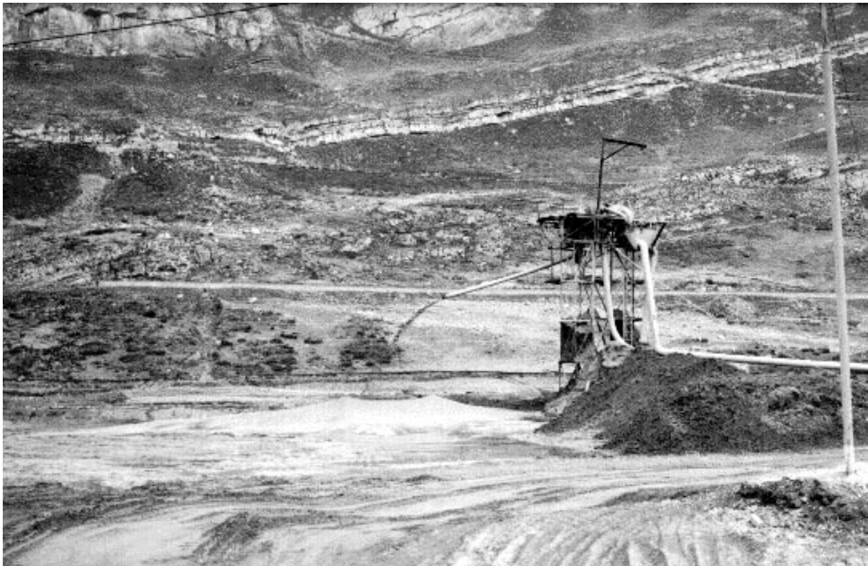
After metals are chemically extracted from ore that has been mined, the resulting wastes are called “tailings.” These tailings in the department of Junín, Peru, are a threat to nearby water sources and other pasture lands. (credit: Chris Hufstader/Oxfam America)
